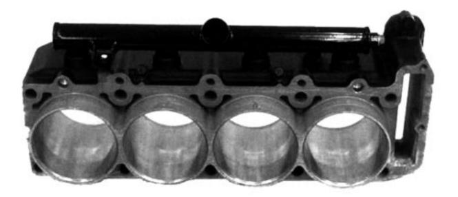
The larger bore and stroke require a new crankshaft with more inertia to work with the larger pistons and crankcases. The pitch between the cylinders is the same as the ZRX1100, but the cam chain sits 3mm further outward to avoid the larger bore and the clutch side is 2mm wider. The total engine width increases only 5mm.
