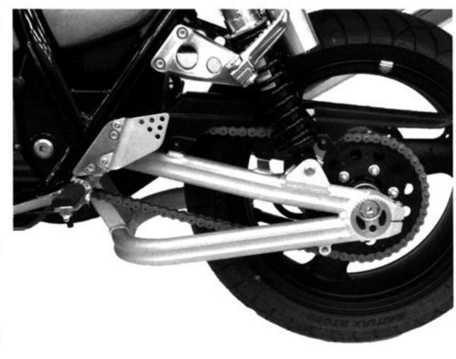
The lower shock mount is moved 12mm further forward to work with the new swingarm pivot position. The result is better suspension action in all conditions.
