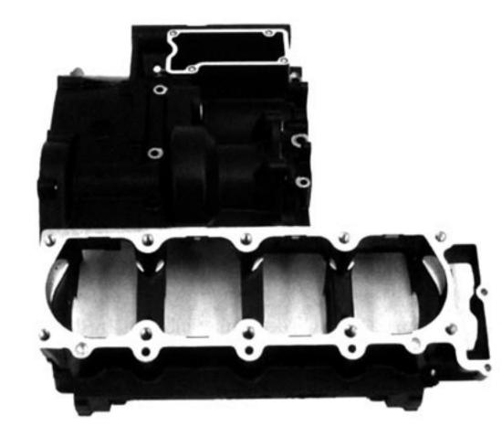
Lubrication is improved with the addition of oil return passages in the cylinder head on the exhaust side between each cylinder. The ZRX1100 used the cam chain galley alone for the oil return.
