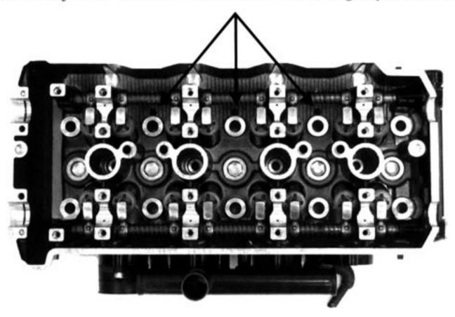
New cam profiles work with the bigger displacement motor for more power with a fat torque curve. The cams are 3mm wider to bridge the larger cylinders.
