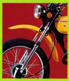
travel Ceriani-type forks for road or rough stuff, with rubber dust shields. Steel rims and trials tires for versatility. Five-way adjustable rear shocks and easy-to-remove, easy-to-service air cleaner. Readily detachable fuel tank. This is the machine that'll run and run with a minimum of maintenance.
