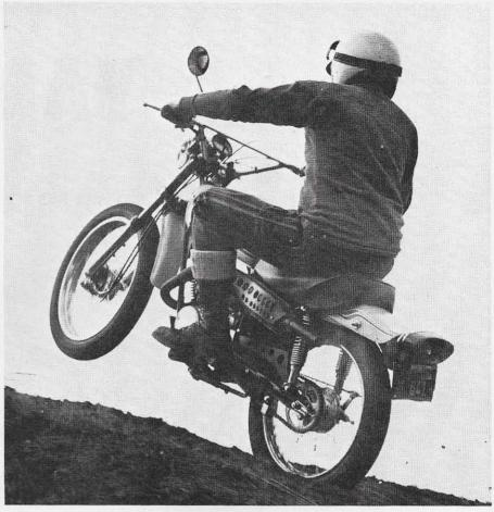
ENGINE Type Single-cylinder two-stroke Bore and stroke 1.95 x 2.04 inches Displacement 99 cc (6.04 cu. in.) **Compression** Ratio 7:1 Ignition Magneto Carburetion Rotary valve induction Lubrication Oil injection DIMENSIONS Length 76.5 inches Seat height 30 inches Wheelbase 49 inches
