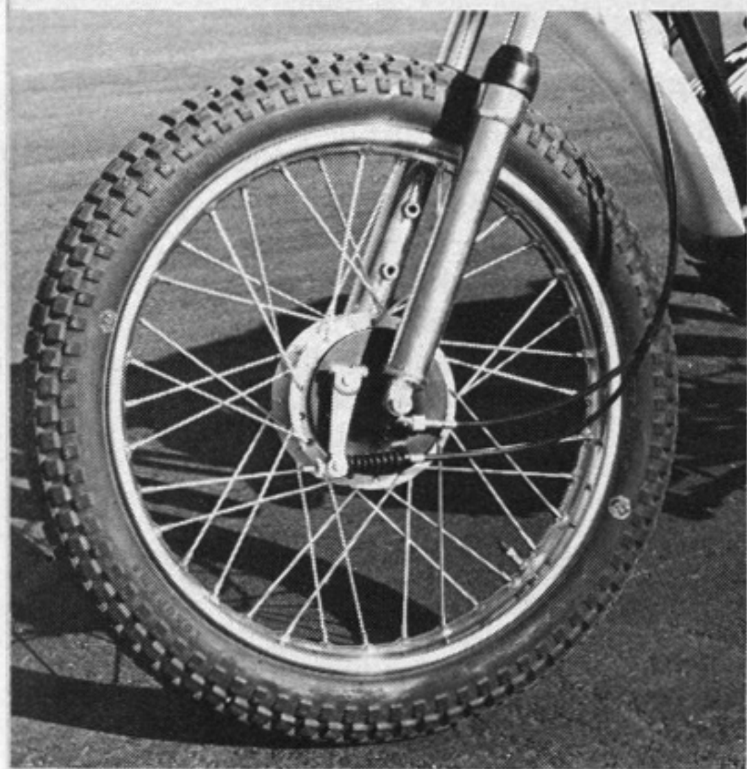
The forks have only limited travel, but deliver good suspension for a trail bike. The front brake hub houses the speedo drive.
