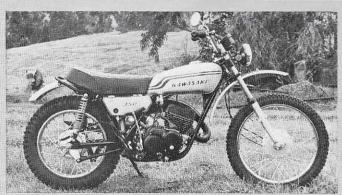
ENGINE Type single cylinder two stroke Bore and stroke 3.17 x 2.68 inches Displacement 346cc **Compression Ratio** 6.8 to 1 Max. Horsepower 33 @ 6,500 rpm Ignition CDI Carburetion rotary valve induction Lubrication automatic oil injection DIMENSIONS
